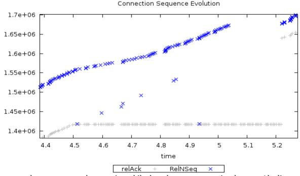
We can see the sequence number growing while the ack sequence remains the same (duplicate acks), until the sequence number stops growing. This is because the sender has filled his perceived space in the receiver window.
