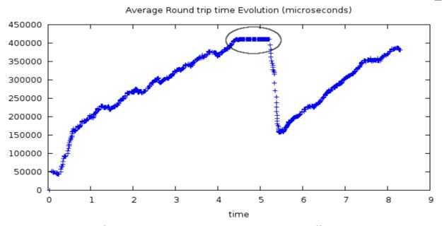
The bottleneck router or firewall in the path has a large output queue buffer and the sender is slowly growing its congestion window exploring the capacity of the path. This growth in congestion window is not increasing the data rate at the receiver, because the output rate from the bottleneck interface remains constant.
