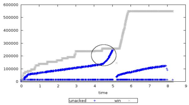
We can see the the receiver is adapting its receive window as the unacked byte count grows, and the average round trip time grows also:
